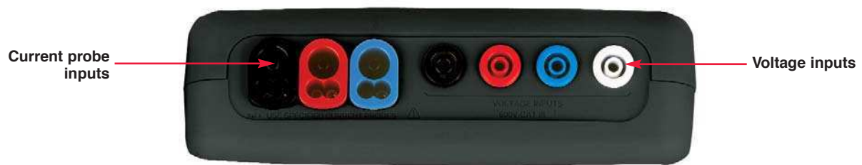
The color-coded input connectors provide dedicated current probe inputs and voltage inputs.
