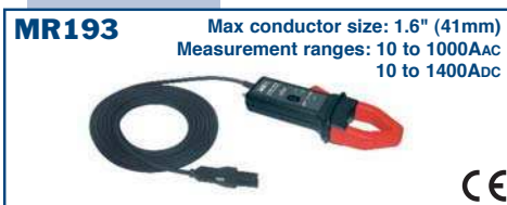
MR193 probe (black connector) (1000Aac/1400Adc) Catalog #2140.28 (10 ft leads)
